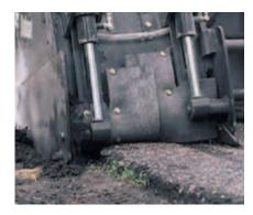
The **ski wear pads** are replaceable and provide consistent depth control by penetrating through debris in the path of travel. Optional planer wheel kit available to replace skis.
