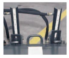
The **depth of the skis** is indicated by a depth gauge visible from the operator seat.
