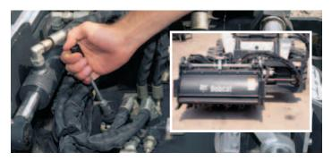
Use the diverter valve control to switch between hydraulic side-shift and hydraulic oscillation.
