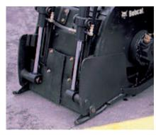
**Dual cylinders**, independently adjustable, provide depth control for each ski.\*\*
